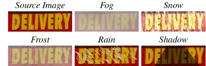
Figure 8. Example images affected by Weather data augmentation.
