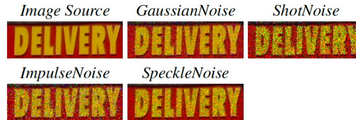
Figure 6. Examples of images affected by Noise data augmentation.
