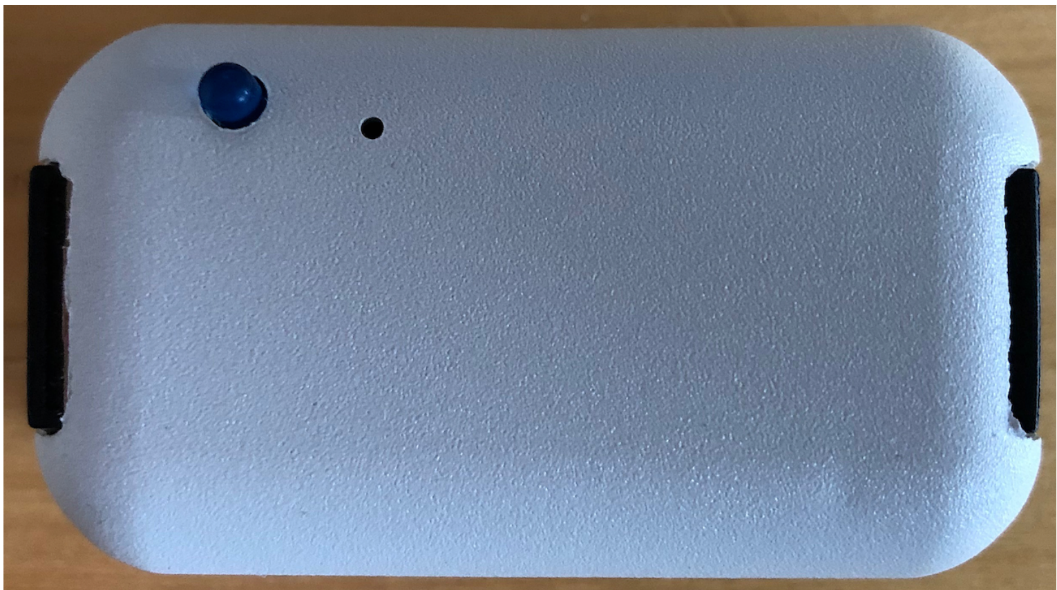
Top of the assembled unit with a pin-hole to allow enabling of the WiFi/Bluetooth pairing.
