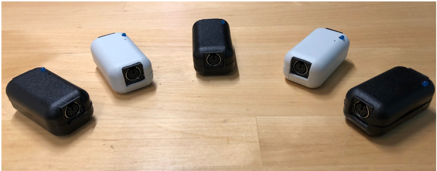
Initial 5 SharpKeys destined for my own computers, together with 2 modified mz25key units (a small internal change allows an mz25key to run the SharpKey firmware) provides keyboard and mouse functionality to all the machines.
