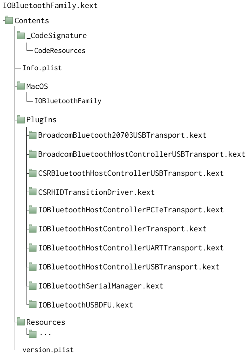
Figure 2.3: Structure of the IOBluetoothFamily.kext.
