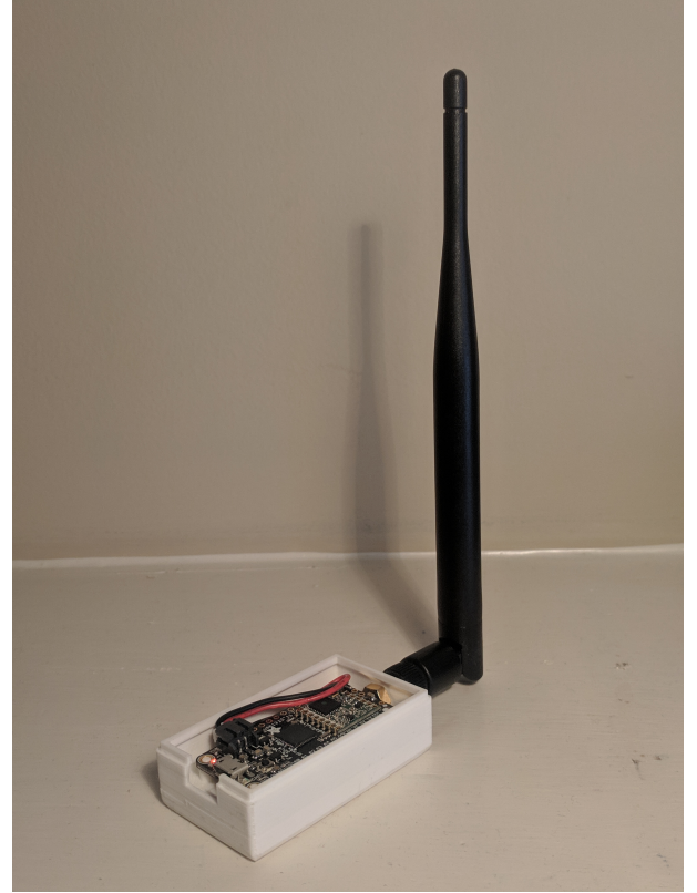
Fig. 2. MeasureMesh Node, with enclosure, battery and antenna.
