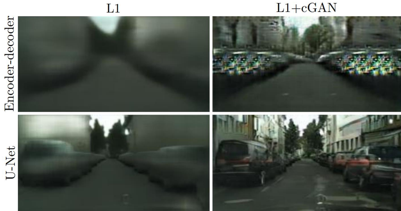
Fig. Adding skip connections to an encoder-decoder to create a “U-Net” results in much higher quality results.
